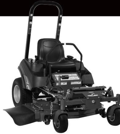
**TYPE:** Mid mount, zero turn, twin stick steering rider with suspension
